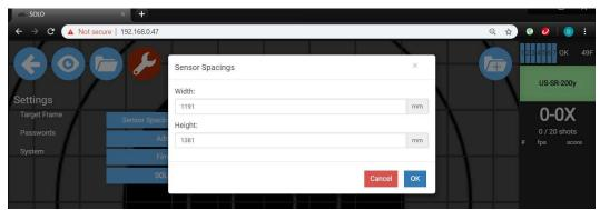
Enter your target sensor width and height. Remember, this data is from left edge to left edge of the upper or lower mics, and top to top of the side mics.
