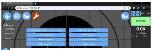
The **Tools** Menu looks like a wrench and is where you will perform a number of maintenance functions such as frame sensor spacing, calibration, optional passwords, update firmware, data maintenance, target name, and WIFI channel.
